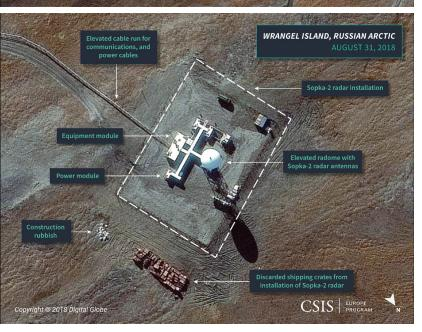
the location of the Sopka-2 is below the peaks of the island's Gora Sovetskaya mountain to the west and northwest, which results in some terrain masking to avoid potential low- and medium-altitude threats from that direction. The significance of this limitation is unclear as the area to the west may be covered by other radar systems.<sup>20</sup>
